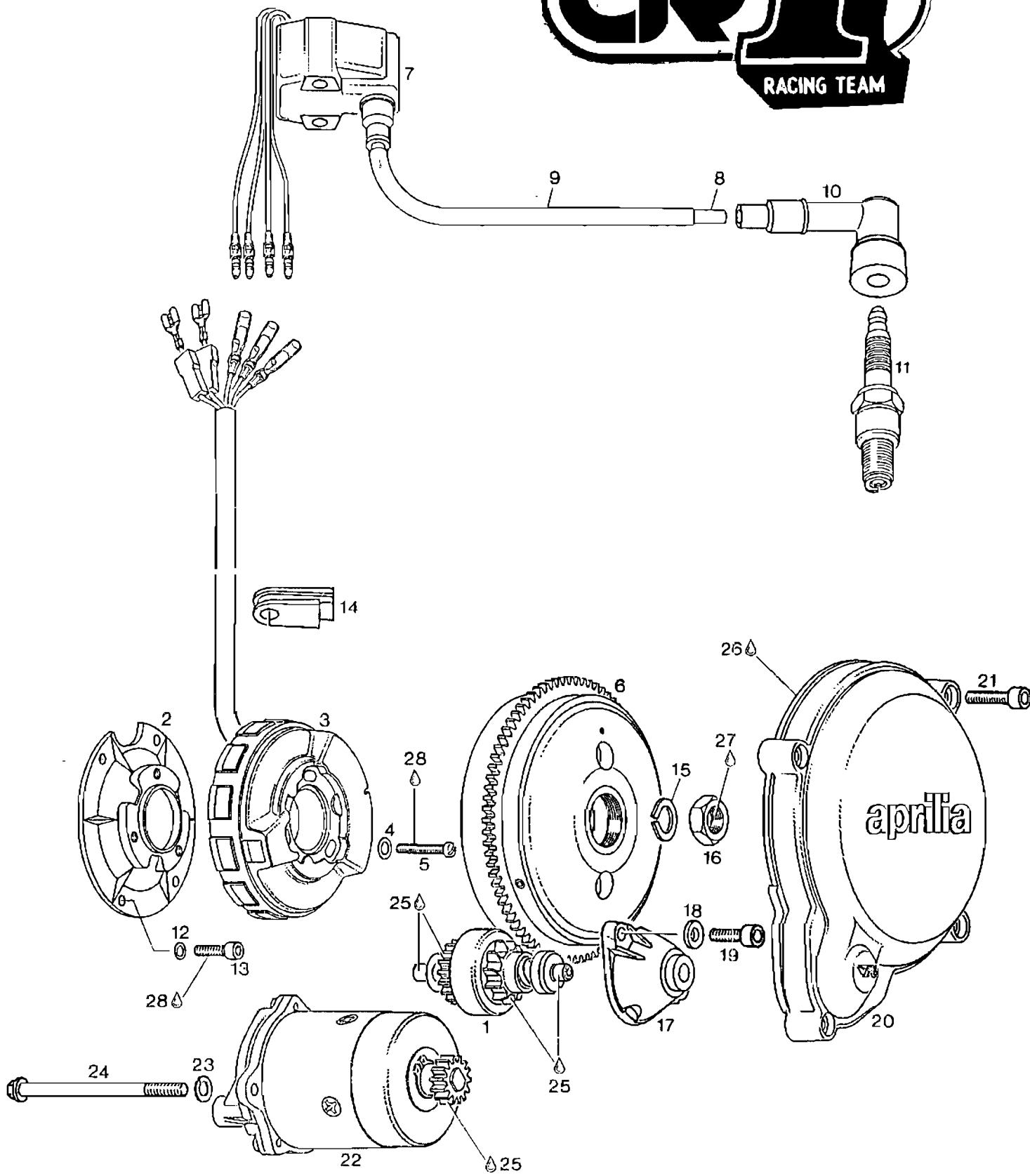
SEM MAGNETZUENDER-GENERATOR, ELEKTROSTARTER,
