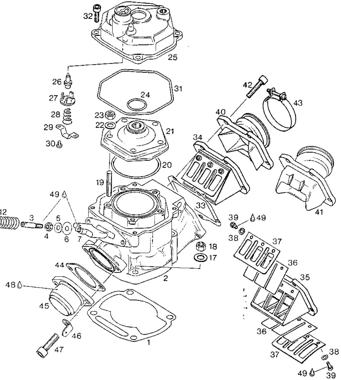
ZYLINDER, AUSPUFFSCHIEBER, ZYLINDERKOPFDECKEL
